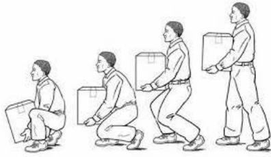
Fig. 5: The squat-lift. From. From *Simple Solutions – Ergonomics for Construction Workers*, NIOSH<sup>6</sup>
